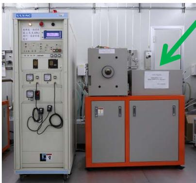
Ulvac E-Beam Evaporator
